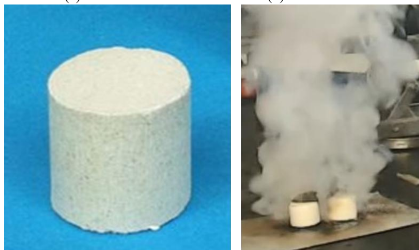
Figure 3: (a) Smoke pellet, and (b) Flameless smoke produced by burning smoke pellet
