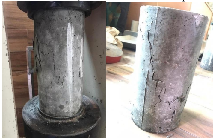
Figure 9: Cylinder placed in machine for split tensile test and after test specimen failure
