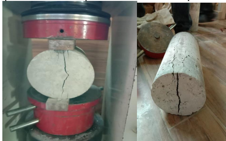
Figure 6: Cylinder placed in machine for split tensile test and after test specimen failure
