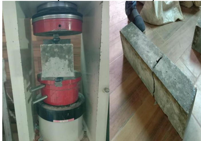
Figure 8: Beam placed in machine for split tensile test and after test specimen failure
