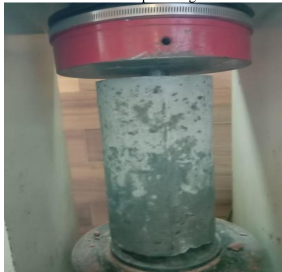
Figure 5: Cylinder before and after test for double punching test
