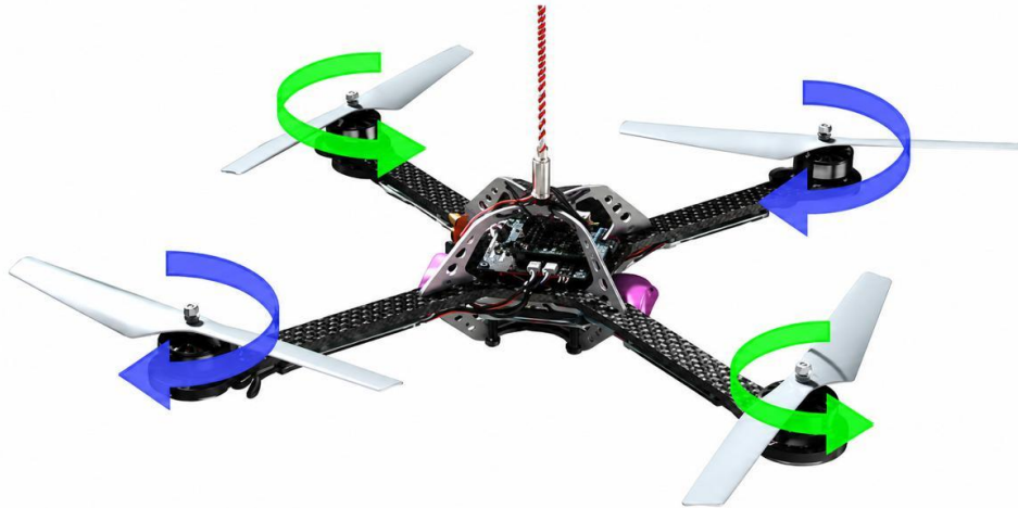
Fig. 1. Quadrotor — AscTec Hummingbird X-configuration platform.
